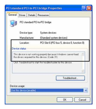
Look for the "Error Code" in the box in the center of the Properties Window and then go to the <u>Windows Error Code</u> section for information on how to resolve this issue.
